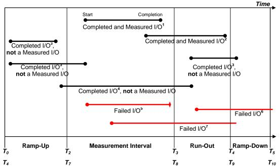
**Completed and Measured I/O<sup>1</sup>**: I/O started and completed within the Measurement Interval. **Completed and Measured I/O<sup>2</sup>**: I/O started within the Measurement Interval and completed within Ramp Down. **Completed I/O<sup>3</sup>**: I/O started before or after the Measurement Interval – not measured. **Completed I/O<sup>4</sup>**: I/O started before and completed after the Measurement Interval – not measured. **Failed I/O<sup>5</sup>**: Signaled as failed by System Software.
