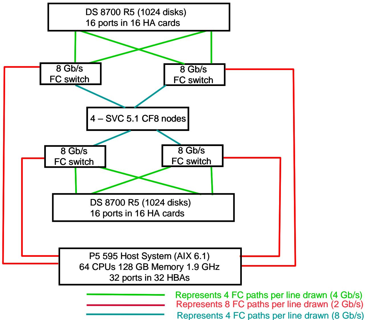
All storage was managed by each SVC node (single image). Each switch had 24 ports enabled, with one zone for node-to-storage traffic and one zone for node-to-host traffic.
