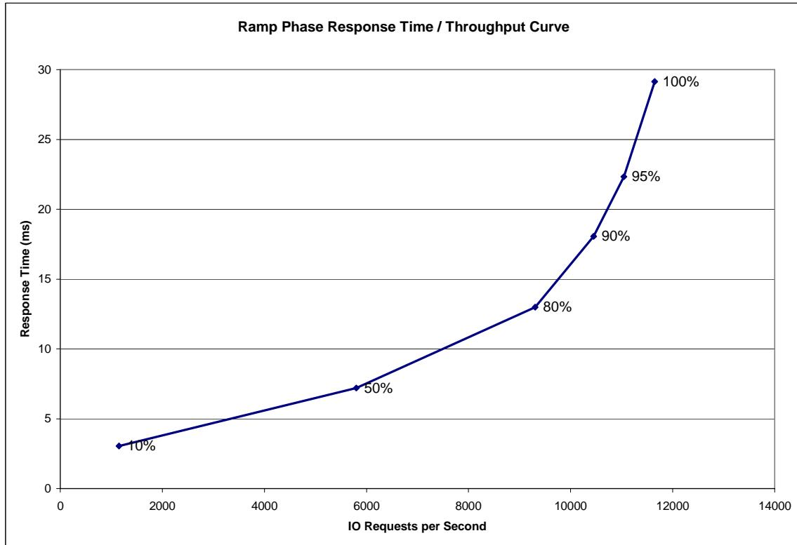
The Response Time-Throughput Curve illustrates the Average Response Time (milliseconds) and I/O Request Throughput at 100%, 95%, 90%, 80%, 50%, and 10% of the workload level used to generate the SPC-1 IOPS™ metric.
