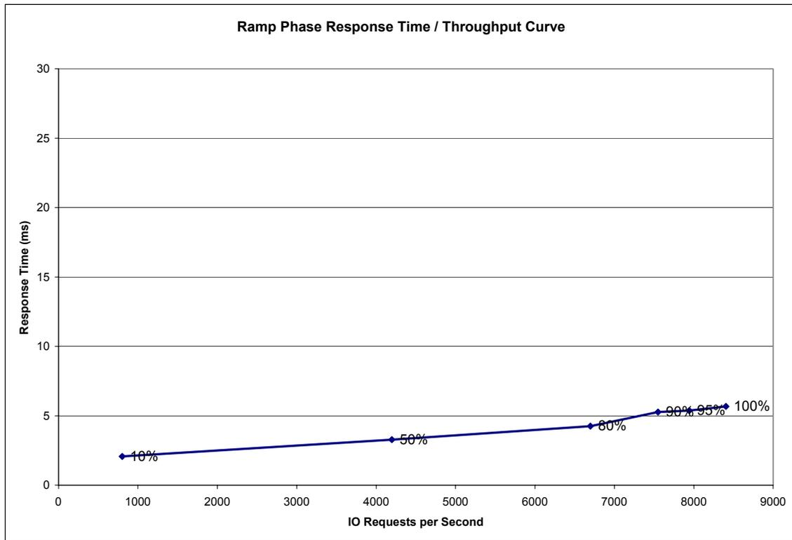
The Response Time-Throughput Curve illustrates the Average Response Time (milliseconds) and I/O Request Throughput at 100%, 95%, 90%, 80%, 50%, and 10% of the workload level used to generate the SPC-1 IOPS™ metric. The SPC-1
