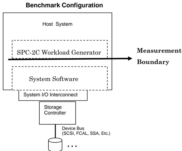
**Figure 5-2: Measurement Boundary in an UNIX System Implementation**
