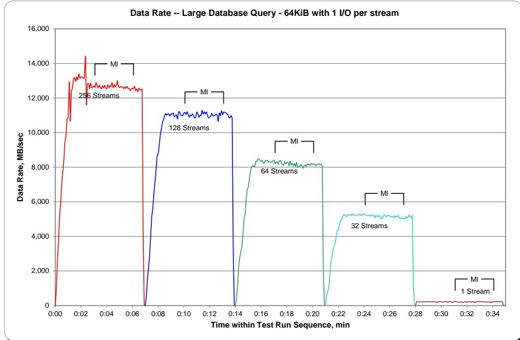
**SPC-2 “Large Database Query/64 KiB Transfer Size/1 Outstanding I/O” Average Data Rate Graph – Measurement Interval (MI) Only**
