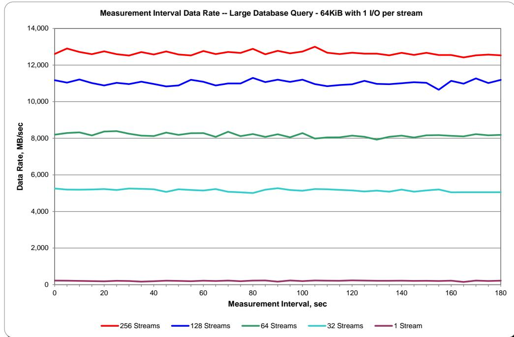
**SPC-2 “Large Database Query/64 KiB Transfer Size/1 Outstanding I/O” Average Data Rate per Stream Graph**
