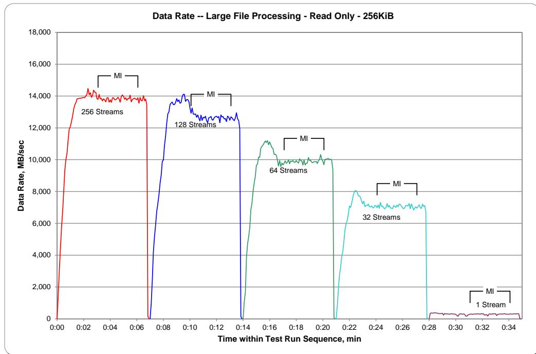
**SPC-2 “Large File Processing/READ ONLY/256 KiB Transfer Size” Average Data Rate Graph – Measurement Interval (MI) Only**
