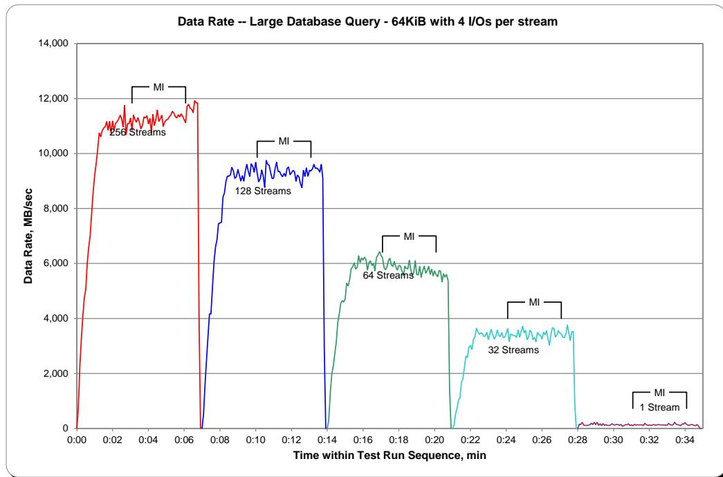
**SPC-2 “Large Database Query/64 KiB Transfer Size/4 Outstanding I/Os” Average Data Rate Graph – Measurement Interval (MI) Only**
