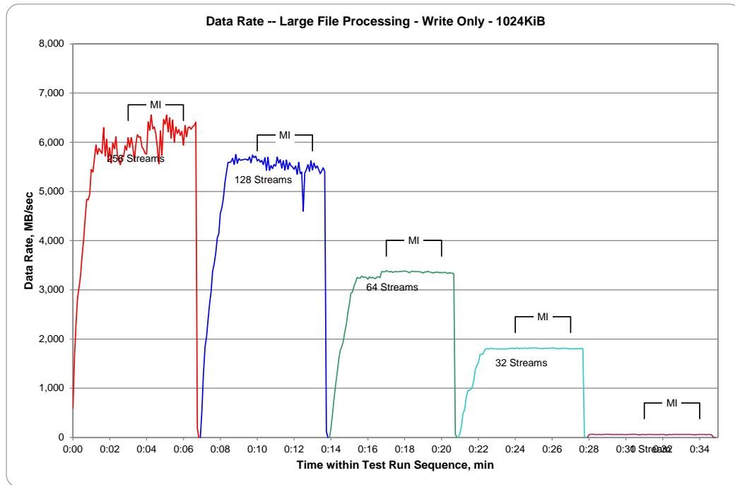
**SPC-2 “Large File Processing/ WRITE ONLY /1024 KiB Transfer Size” Average Data Rate Graph – Measurement Interval (MI) Only**
