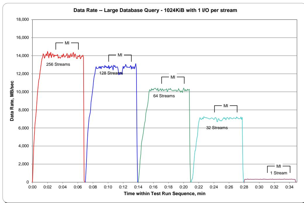
**SPC-2 “Large Database Query/1024 KiB Transfer Size/1 Outstanding I/O” Average Data Rate Graph – Measurement Interval (MI) Only**
