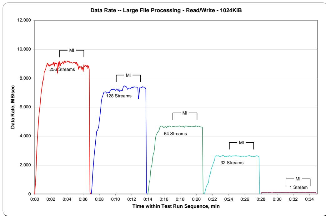
**SPC-2 “Large File Processing/ READ-WRITE/1024 KiB Transfer Size” Average Data Rate Graph – Measurement Interval (MI) Only**
