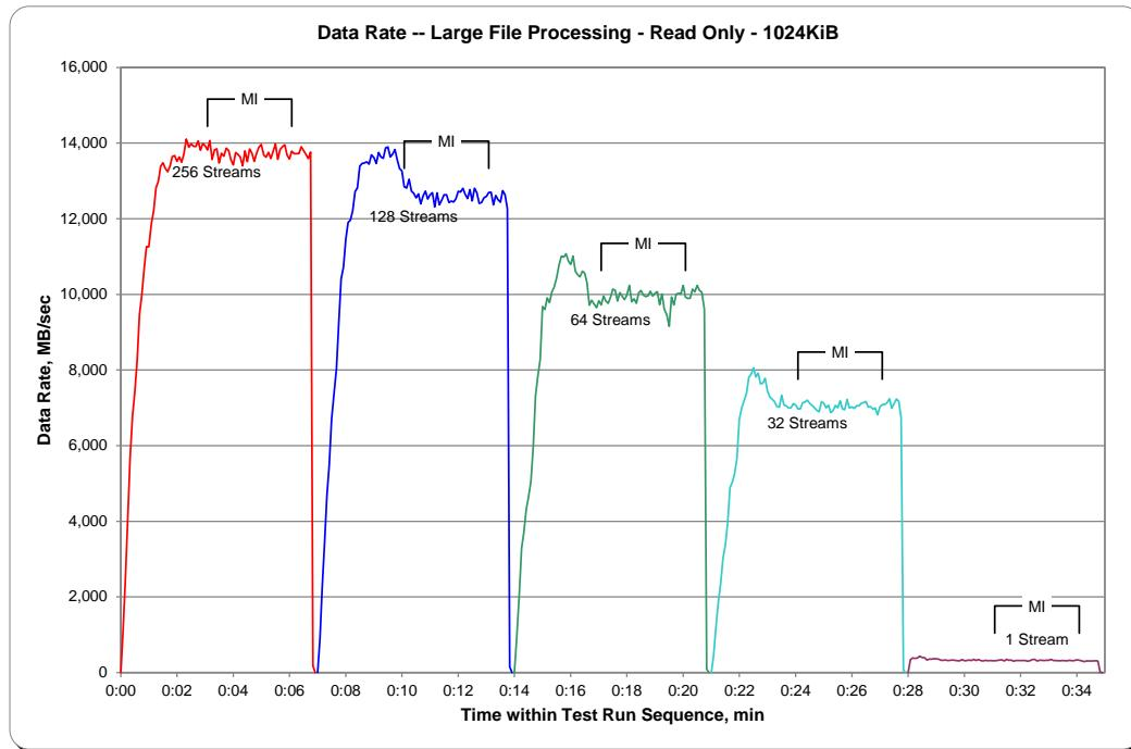
**SPC-2 “Large File Processing/READ ONLY/1024 KiB Transfer Size” Average Data Rate Graph – Measurement Interval (MI) Only**
