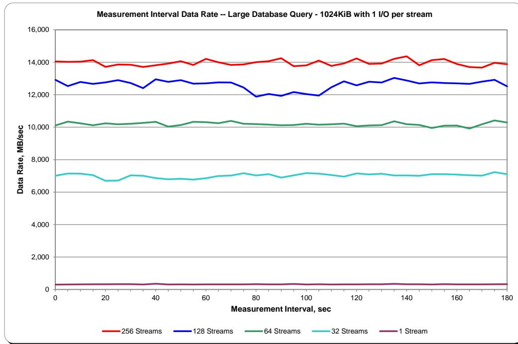
**SPC-2 “Large Database Query/1024 KiB Transfer Size/1 Outstanding I/O” Average Data Rate per Stream Graph**
