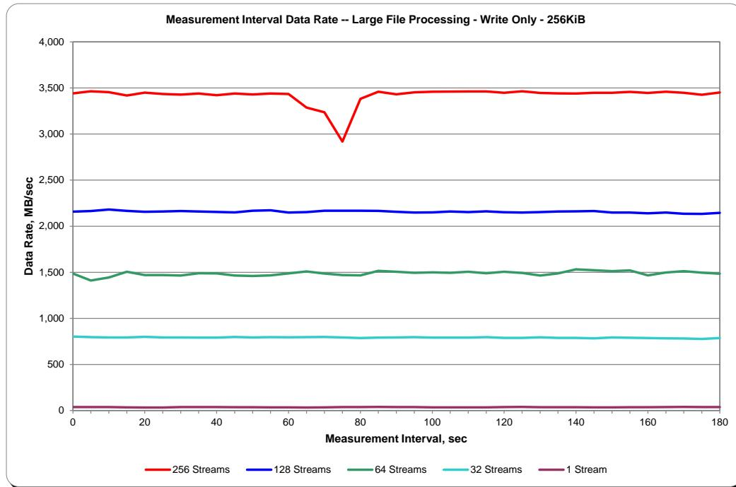
**SPC-2 “Large File Processing/ WRITE ONLY /256 KiB Transfer Size” Average Data Rate per Stream Graph**
