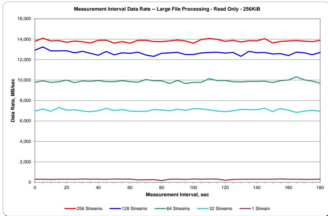
**SPC-2 “Large File Processing/READ ONLY/256 KiB Transfer Size” Average Data Rate per Stream Graph**
