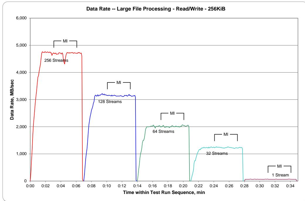
**SPC-2 “Large File Processing/READ-WRITE/256 KiB Transfer Size” Average Data Rate Graph – Measurement Interval (MI) Only**
