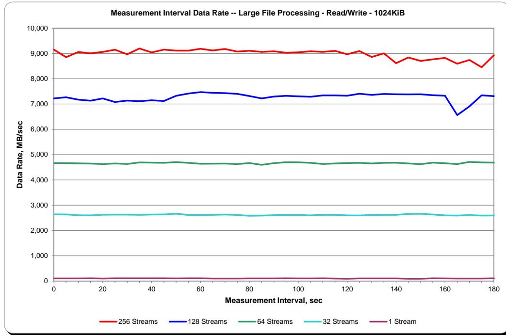
**SPC-2 “Large File Processing/READ-WRITE/1024 KiB Transfer Size” Average Data Rate per Stream Graph**
