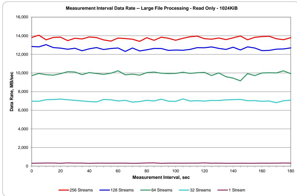
**SPC-2 “Large File Processing/READ ONLY/1024 KiB Transfer Size” Average Data Rate per Stream Graph**
