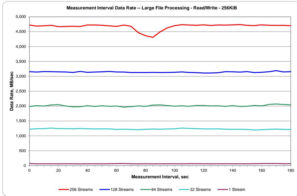
**SPC-2 “Large File Processing/READ-WRITE/256 KiB Transfer Size” Average Data Rate per Stream Graph**
