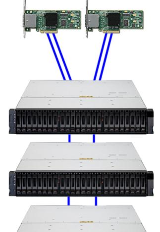
IBM System Storage® DS3524 Express Dual Controller (24 SAS Disk Slots) 20 – 300 GB 10K RPM SAS disk drives
