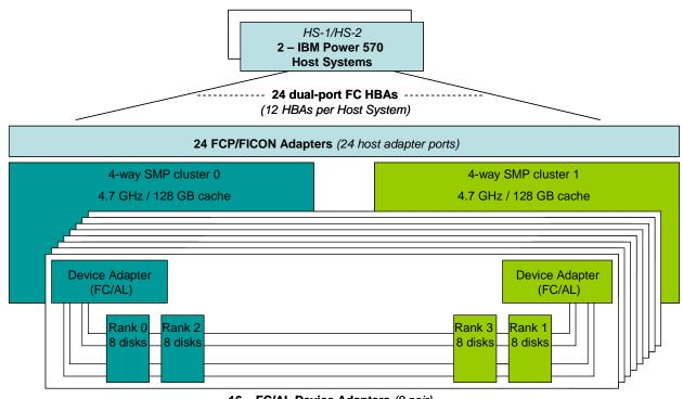
16 – FC/AL Device Adapters (8 pair) 256 – 300 GB 15K RPM Disk Drives
