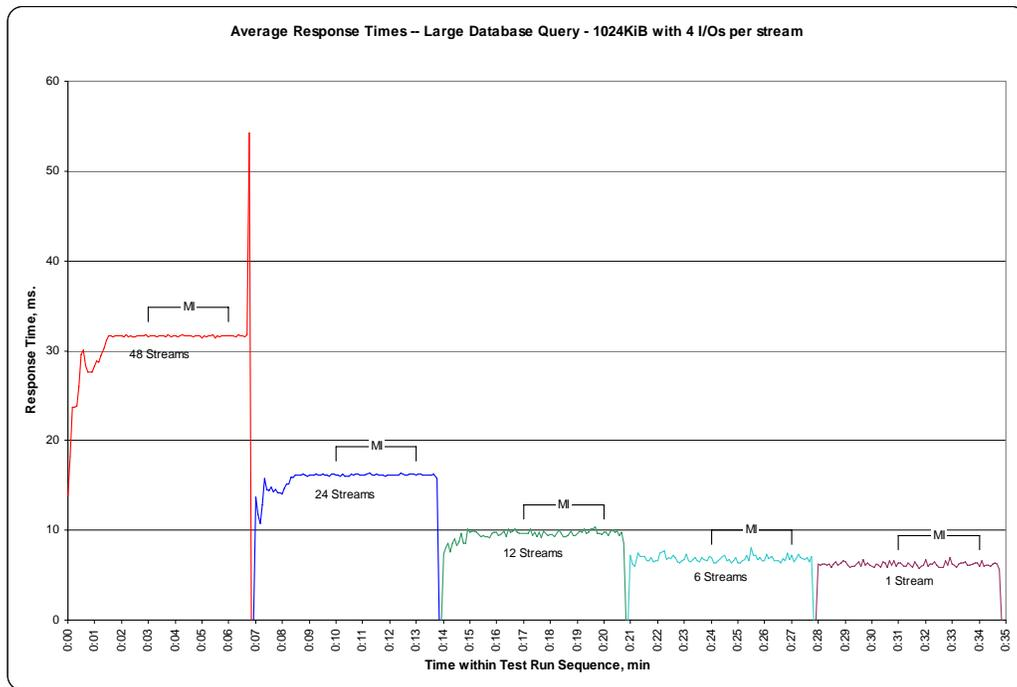
**SPC-2 “Large Database Query/1024 KiB Transfer Size/1 Outstanding I/O” Test Run Data – Ramp-Up Period**
