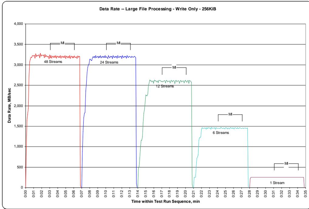
**SPC-2 “Large File Processing/ WRITE ONLY /256 KiB Transfer Size” Average Data Rate Graph – Measurement Interval (MI) Only**
