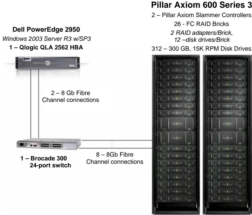
**Host System(s) and Tested Storage Configuration Components**
