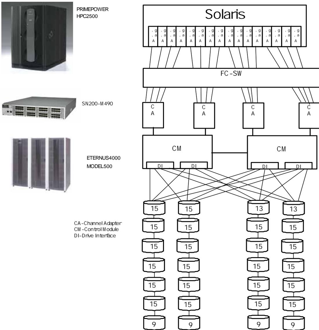
**Benchmark Configuration/Tested Storage Configuration Components**
