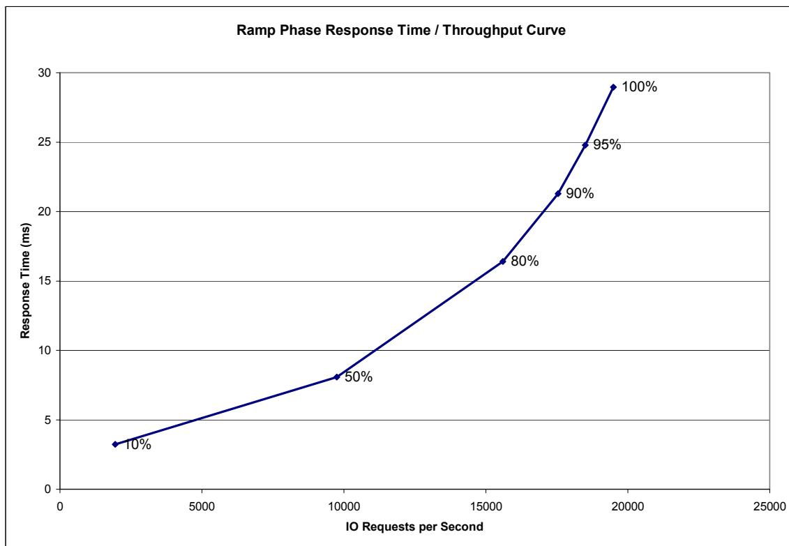
The Response Time-Throughput Curve illustrates the Average Response Time (milliseconds) and I/O Request Throughput at 100%, 95%, 90%, 80%, 50%, and 10% of the workload level used to generate the SPC-1 IOPS™ metric.
